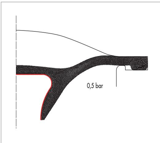
Fig. 17 Diaphragm axially deformed
