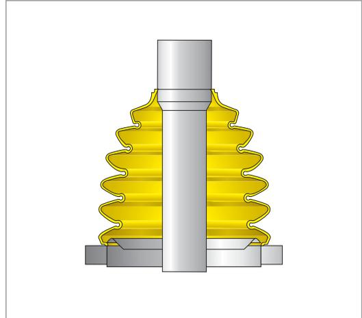
Fig. 14 Bellows installed
