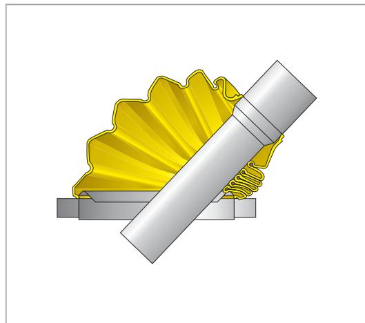
Fig. 15 Bellows deflected and tilted
