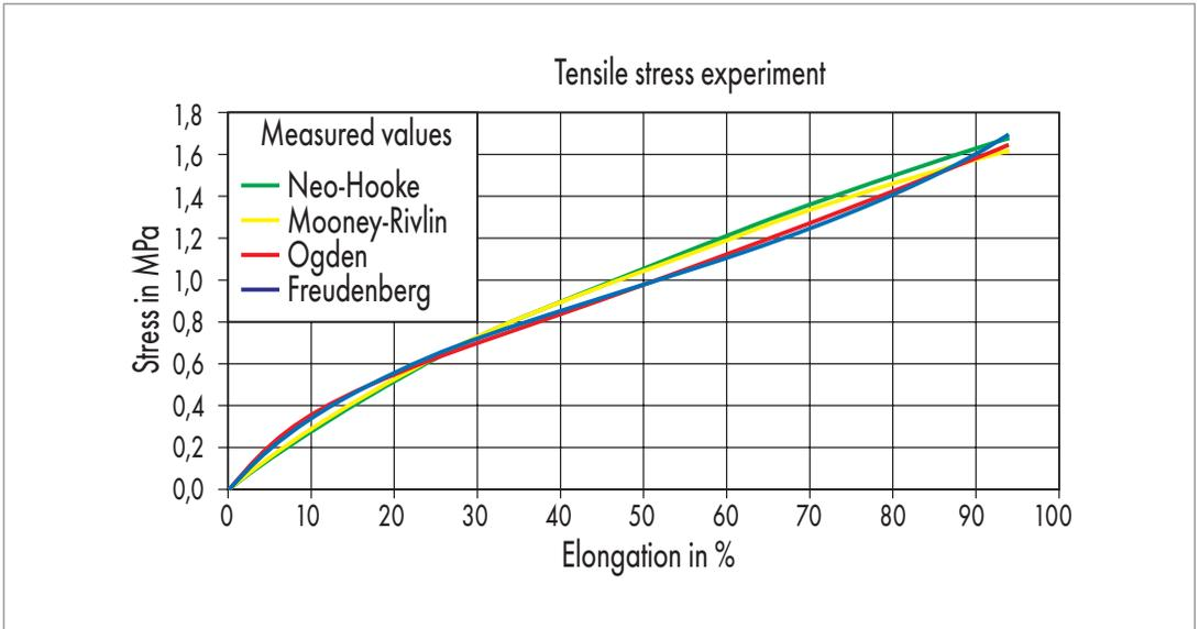
Fig. 2 Material models adapted to a single-axis tensile trial
