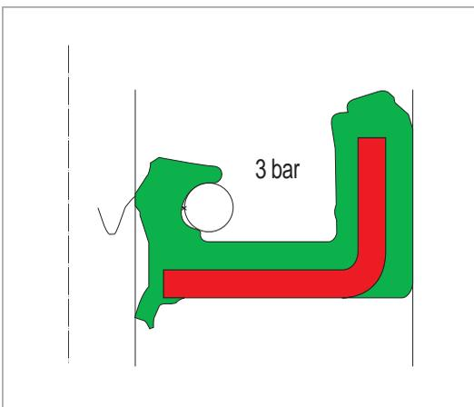
Fig. 5 Simmerring with optimised profile
