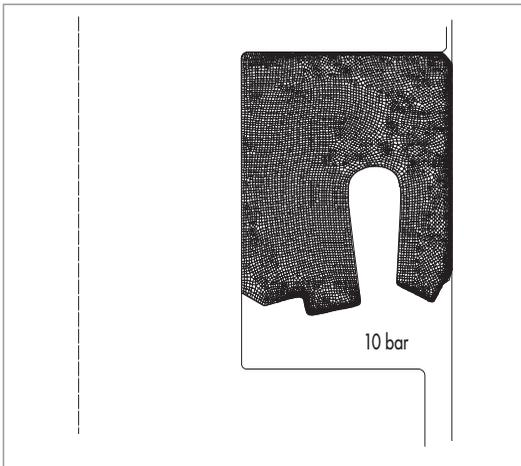
Fig. 9 Merkel U-Ring NAPN 125 deformed 10 bar
