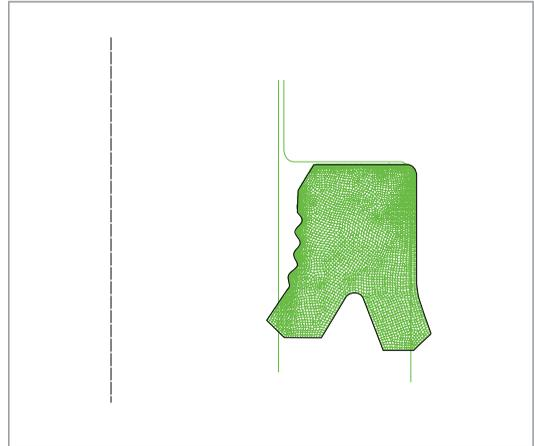
Fig. 6 Merkel U-Ring LF 300 undeformed
