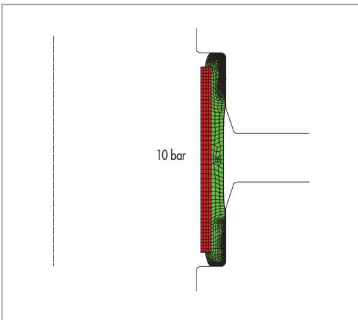
Fig. 13 Plug & Seal plug connection deformed 10 bar
