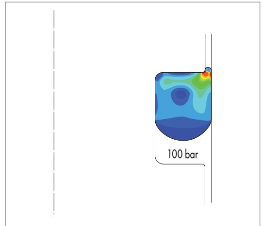
Fig. 11 ISC O-Ring 40-4 100 bar gap extrusion
