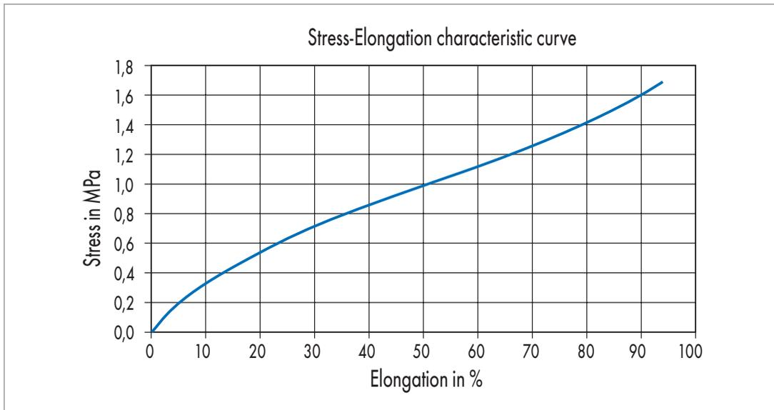
Fig. 1 Tensile trials on an elastomer
