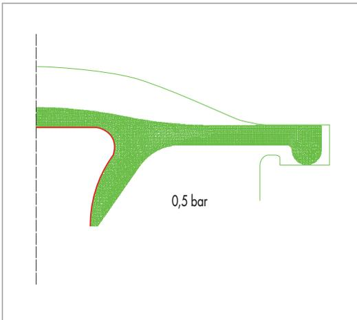
Fig. 16 Diaphragm undeformed
