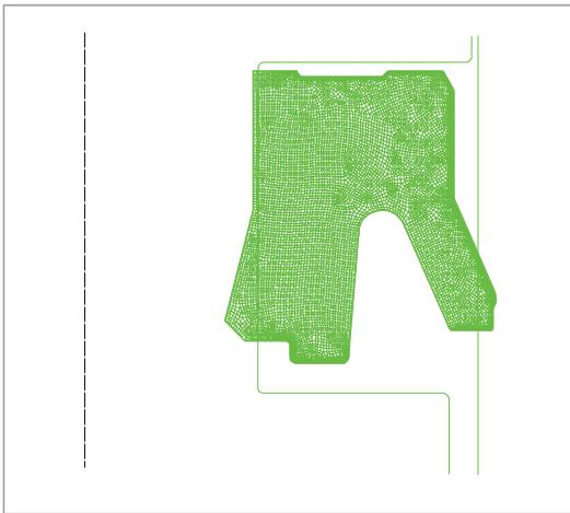
Fig. 8 Merkel U-Ring NAPN 125 undeformed
