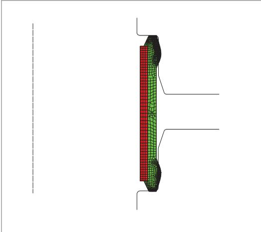
Fig. 12 Plug & Seal plug connection undeformed
