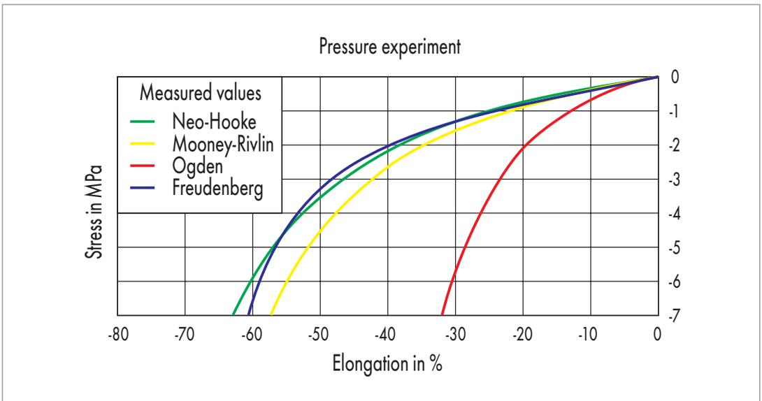
Fig. 3 Material models adapted to a single-axis compressive trial
