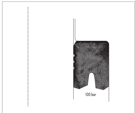
Fig. 7 Merkel U-ring deformed 100 bar
