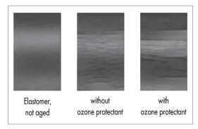
Fig. 2 Damage to elastomer by the effect of ozone
