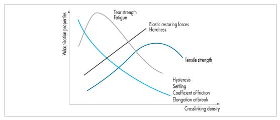
Graph 10 Influence of cross-linking density on the elastomer properties
