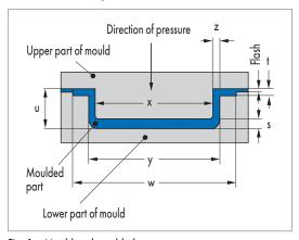
Fig. 1 Mould and moulded part
