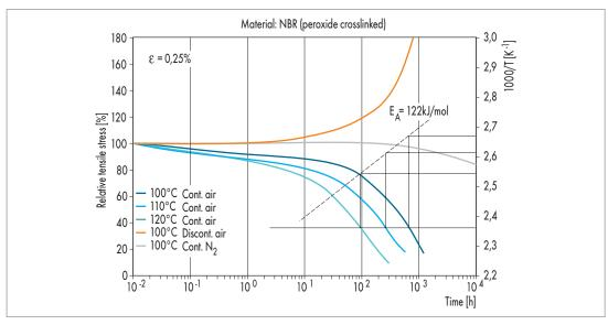
Graph 8 Predicted service life based on extrapolation of measured values of the tensile stress relation (material: NBR wetted with peroxide) measured in air and nitrogen at various temperatures.
