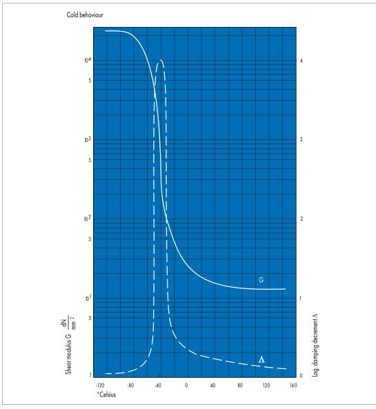
Graph 5 Torsion vibration test in accordance with DIN 53 445. Dynamic shear modulus G and logarithmic decrement  $\Lambda$  of a material from Simrit based on CR
