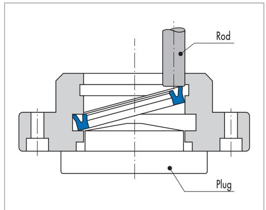
Fig. 24 Fitting aid for rod seals
