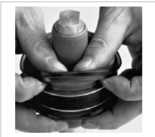
Fig. 26 Snap-in fitting of a piston seal
