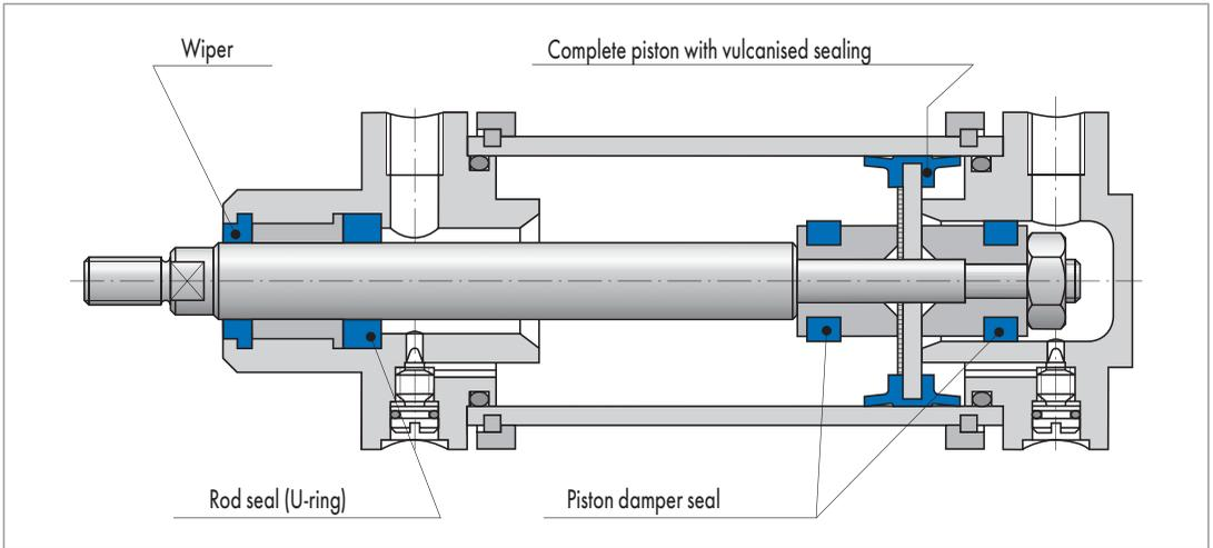
Fig. 3 Pneumatic cylinder II
