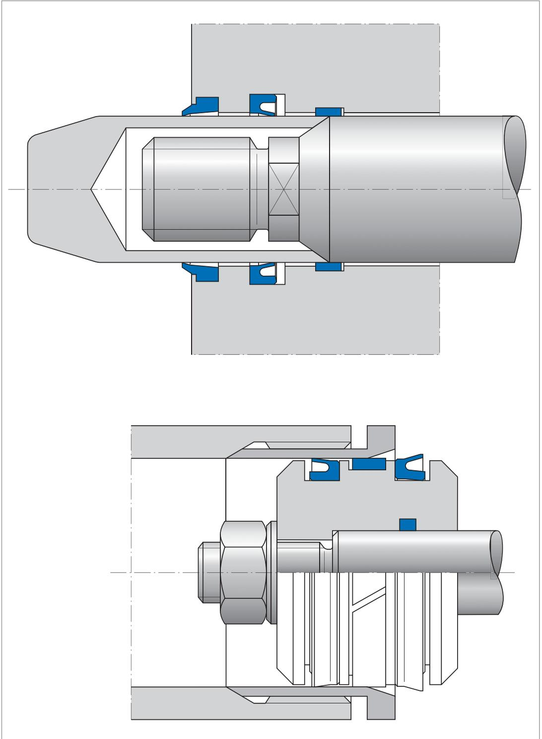
Fig. 19 Covering threads when mounting seals
