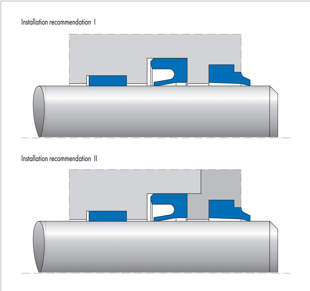
Fig. 20 Fitting types of rod seals
