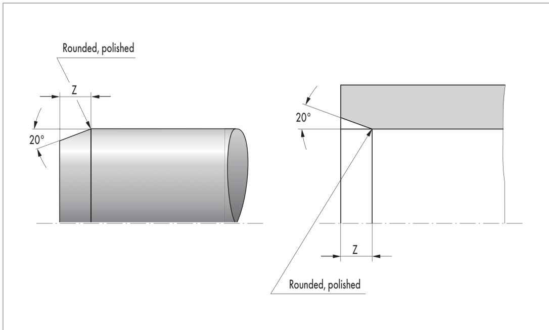
Fig. 18 Chamfering rods and pipes
