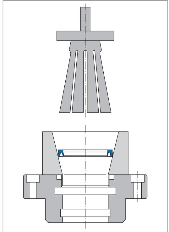
Fig. 23 Fitting of rod seals
