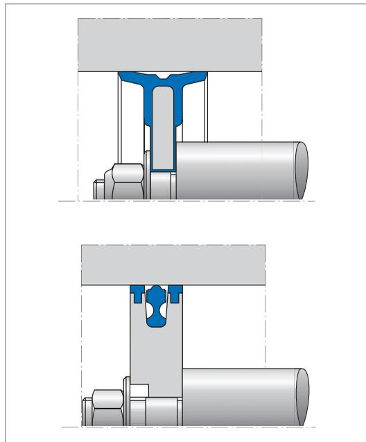
Fig. 28 Assembly of pneumatic complete pistons
