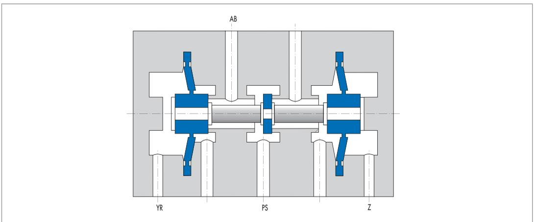
Fig. 8 Pneumatic 5/2-way valve
