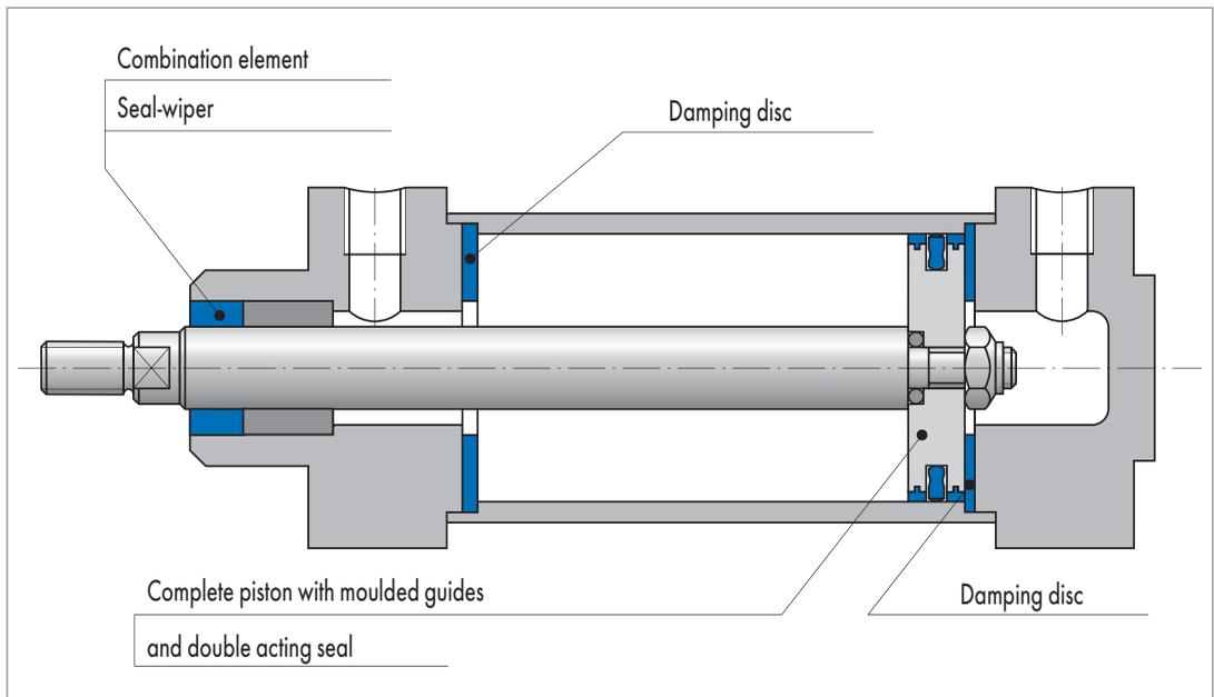
Fig. 1 Pneumatic cylinder I
