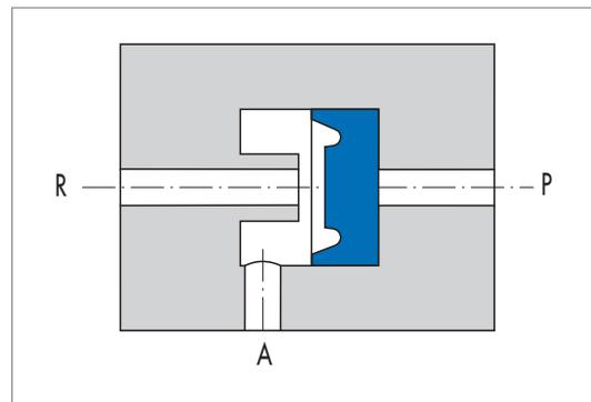
Fig. 6 Pneumatic quick-venting valve
