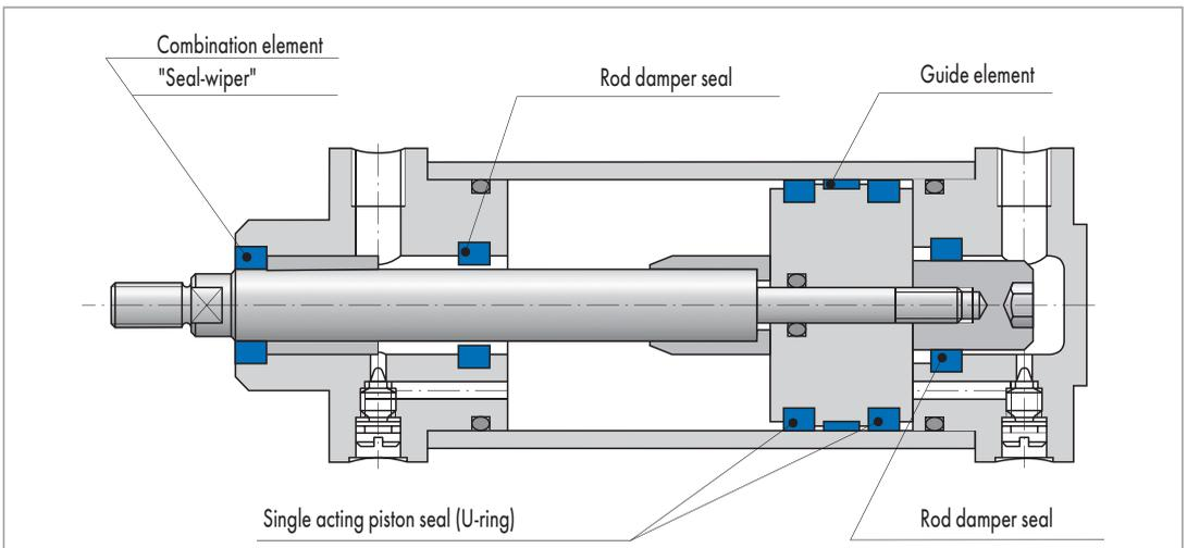
Fig. 4 Pneumatic cylinder III
