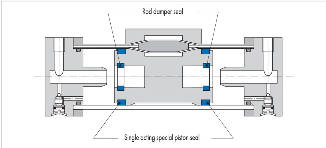
Fig. 5 Pneumatic cylinder without piston rod
