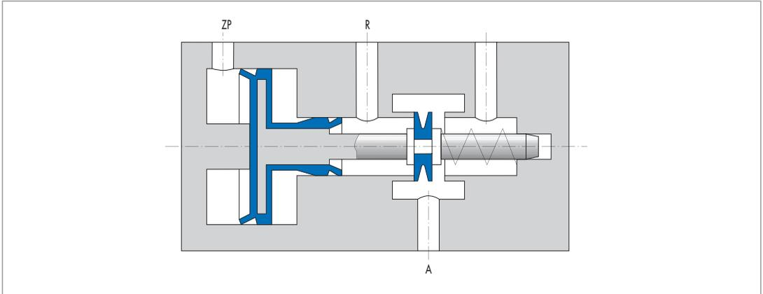
Fig. 7 Pneumatic 3/2-way valve
