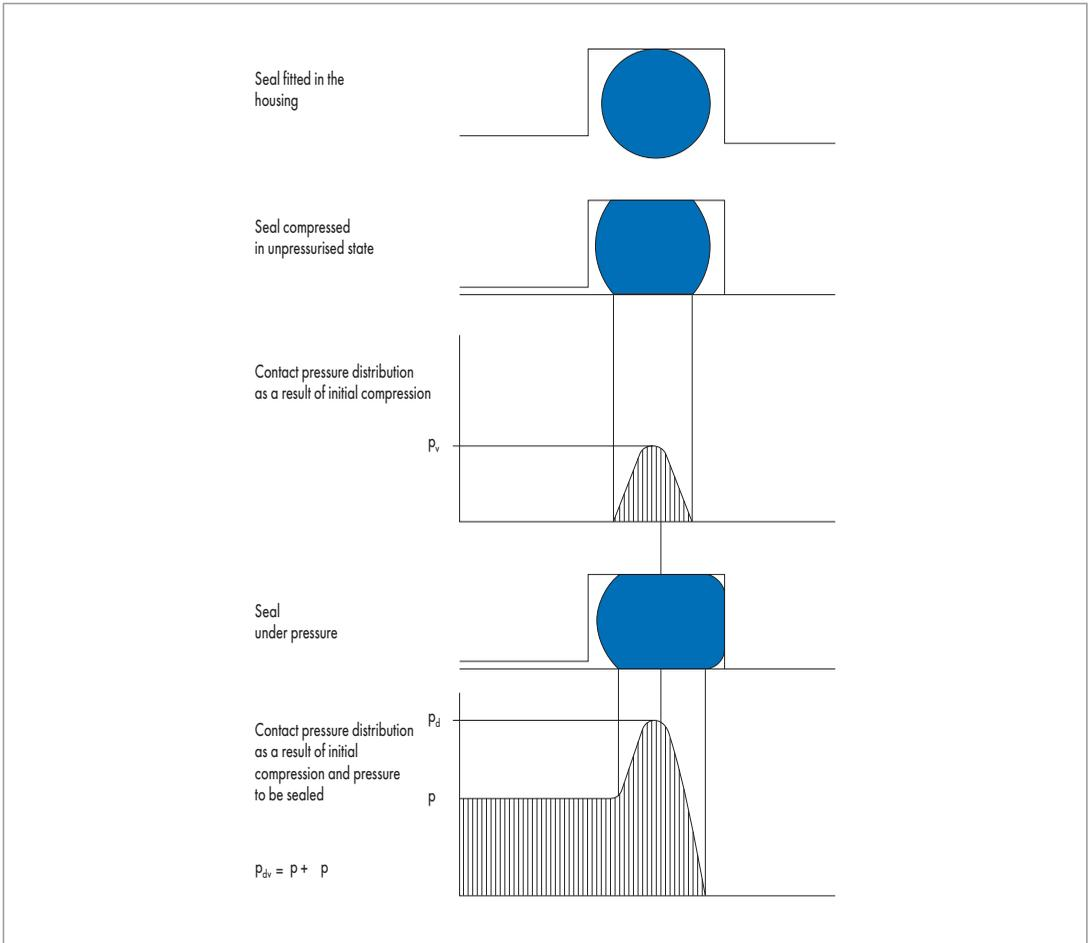
Fig. 9 Automatic sealing effect with elastic seals
