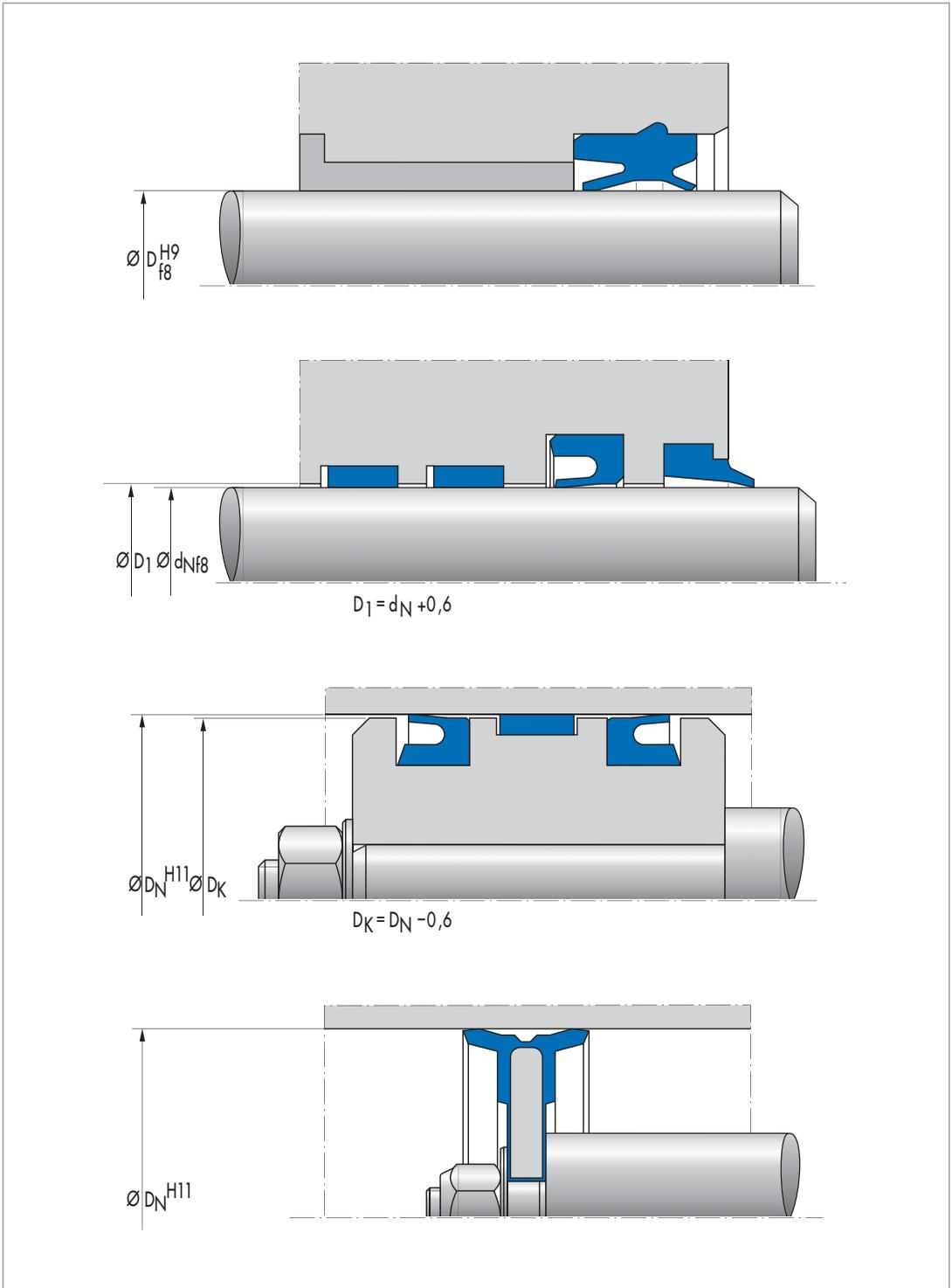
Fig. 16 Fitting and tolerances for seals and guides
