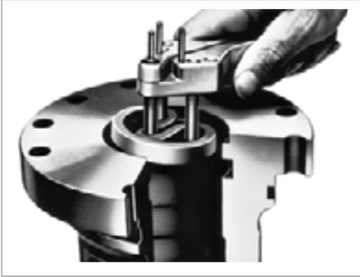
Fig. 21 Fitting tool for rod seals
