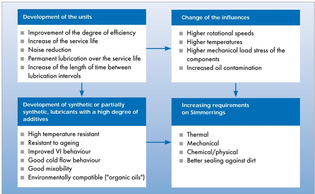
Fig. 18 Increasing requirements on Simmerrings
