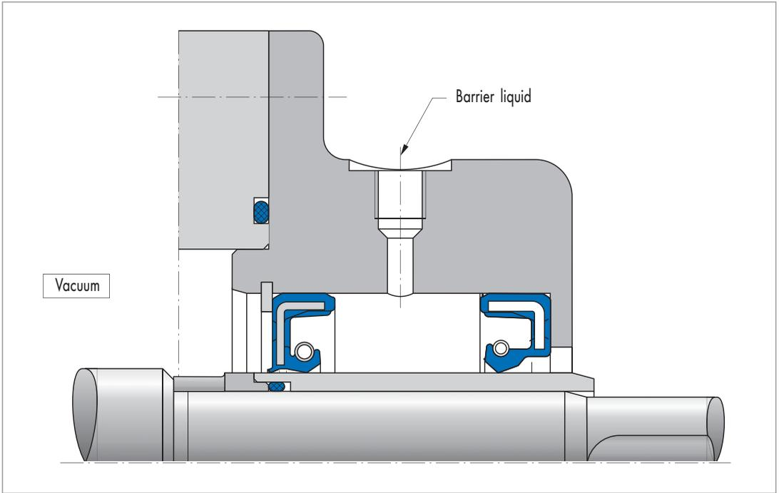
Fig. 7 Sealing against a vacuum
