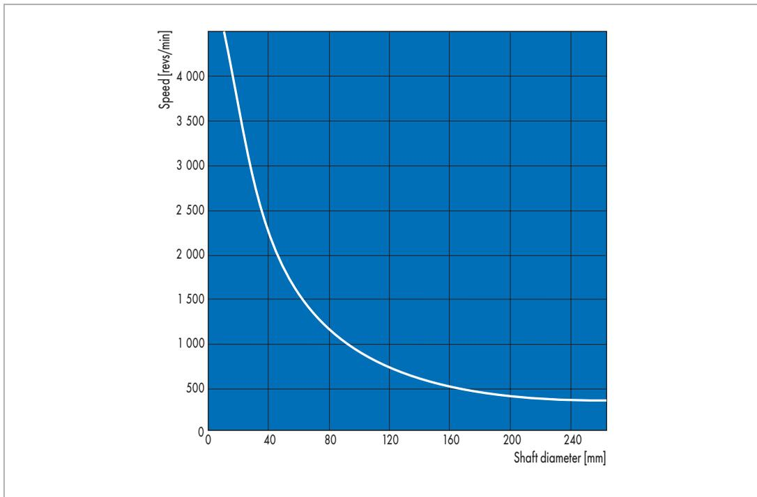
Fig. 28 Permissible rotational speeds with rotating Simmerrings on fixed shafts
