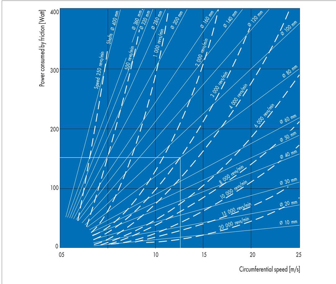
Fig. 15 Recommended values for the friction loss on a Simmerring in engine oil SAE 20, at T=100 °C,
