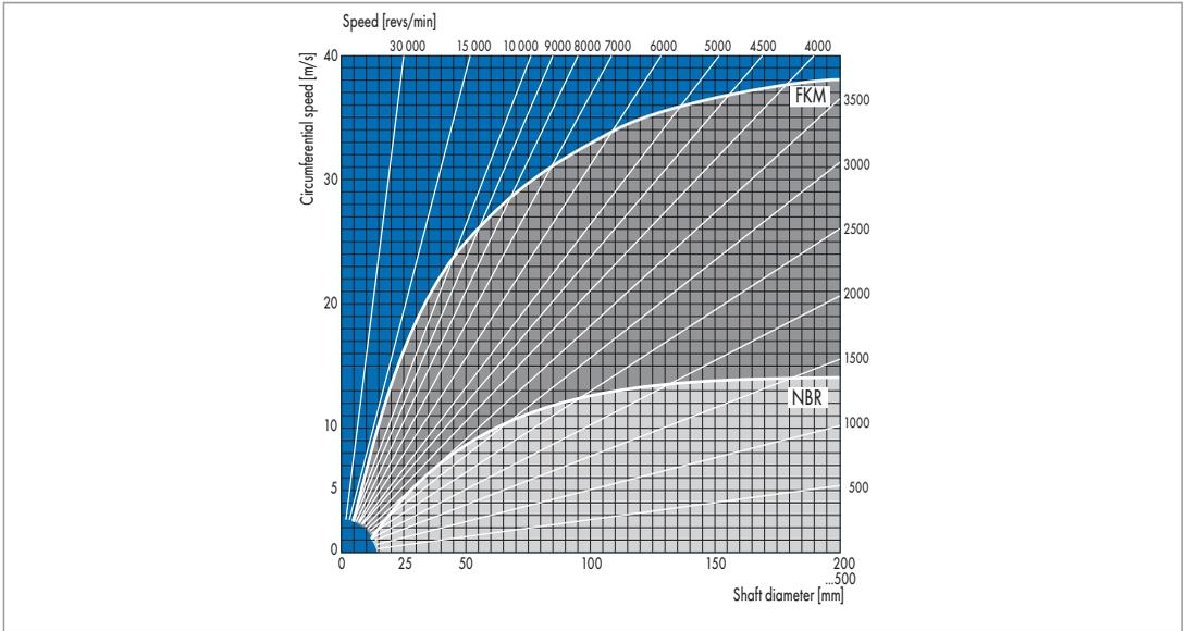
Permissible circumferential speed for Simmerrings made of the material NBR (72 NBR 902) and FKM (75 FKM 585) when sealing engine oil SAE 20. Usage of Simmerring with SL (dust lip):  $v = \max. 8 \text{ m/s}$ .
