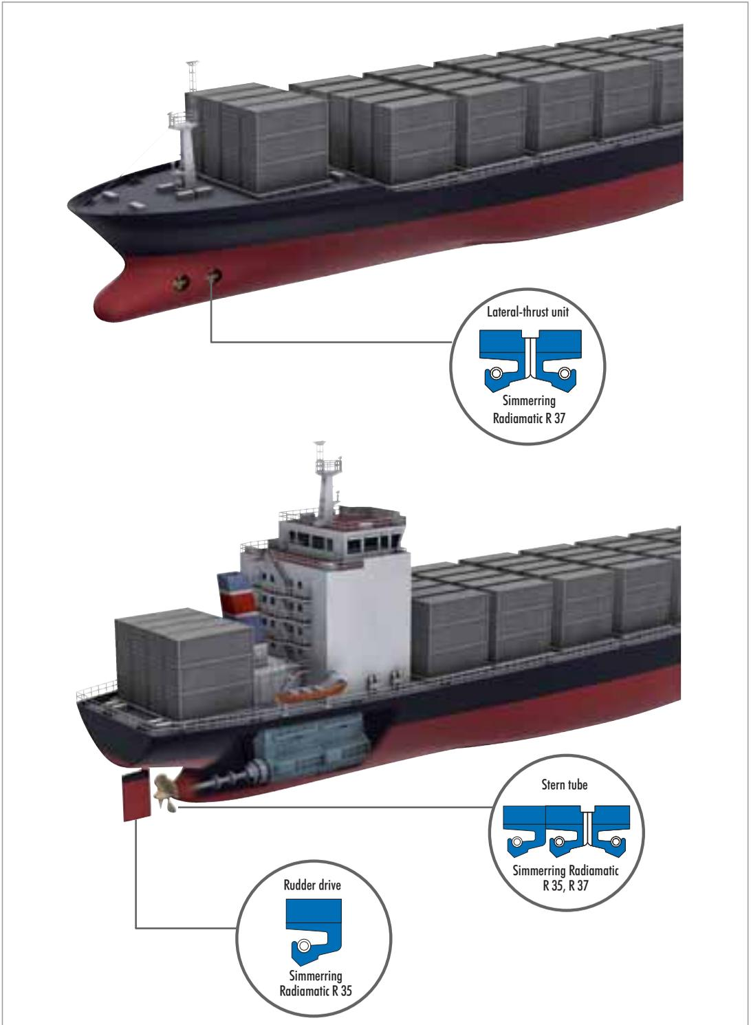
Fig. 5 Simmerrings in marine technology for underwater applications
