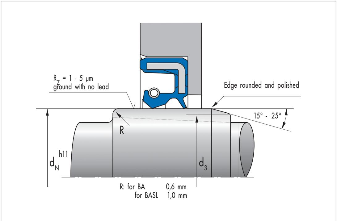
Fig. 34 Radius and chamfering of shaft
