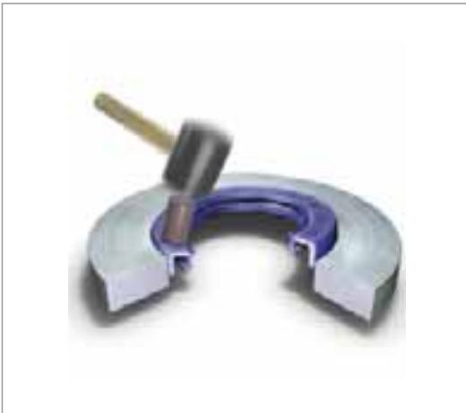
Fig. 47 Inclined fitting not permissible
