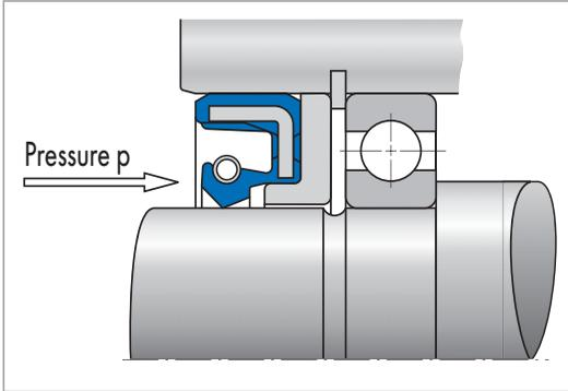
Fig. 26 Installation of a Simmerring with back-up ring
