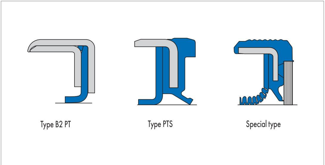
Fig. 36 Simmerrings with PTFE sealing lip
