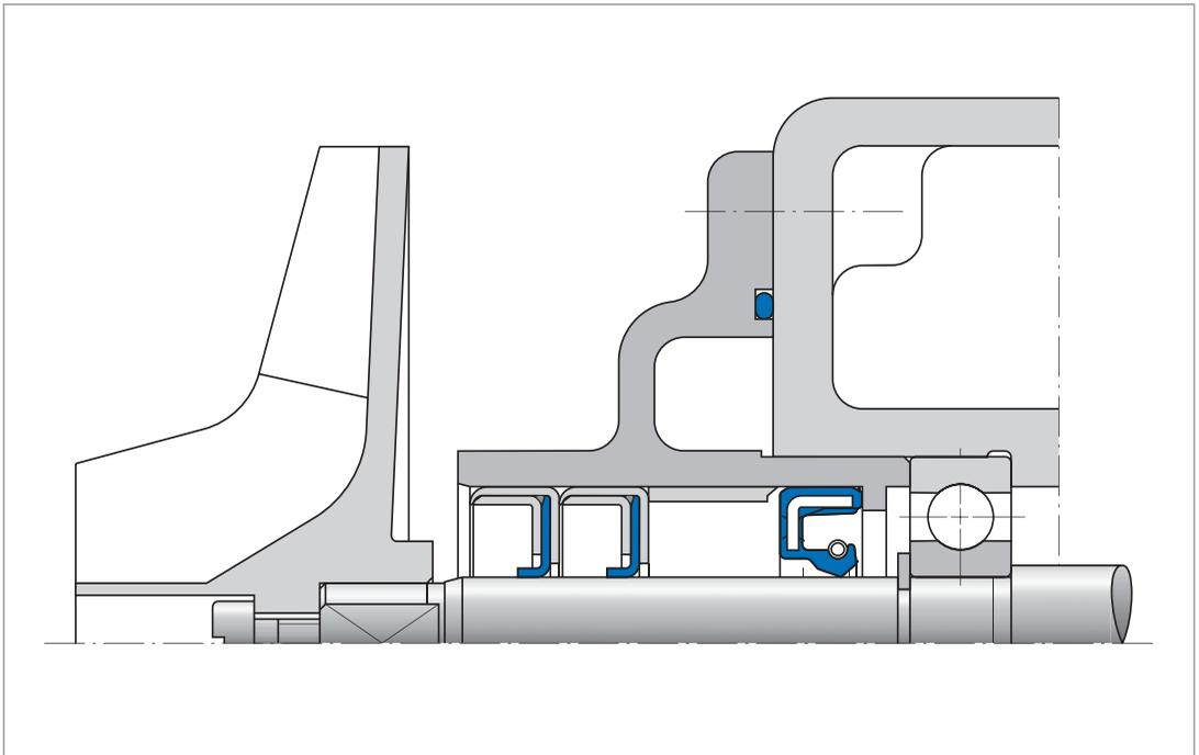
Fig. 8 Sealing against aggressive media (Example: pumps)
