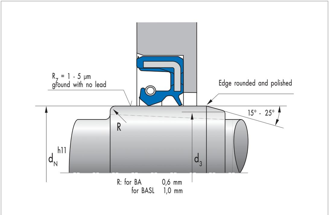
Fig. 34 Radius and chamfering of shaft
