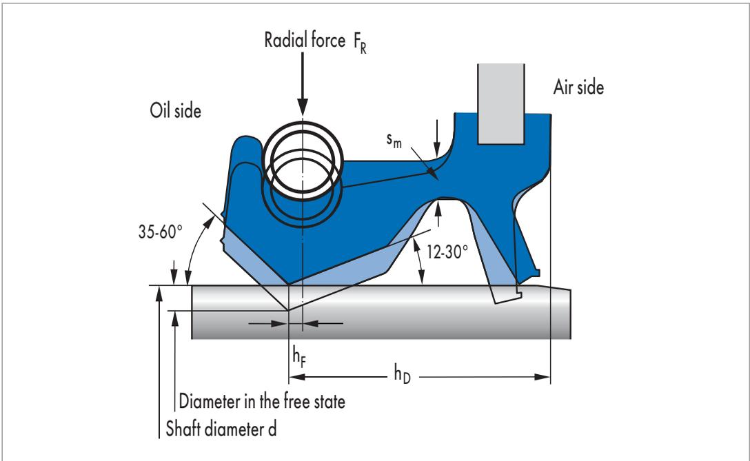
Fig. 11 Dimensions of the sealing lip profile
