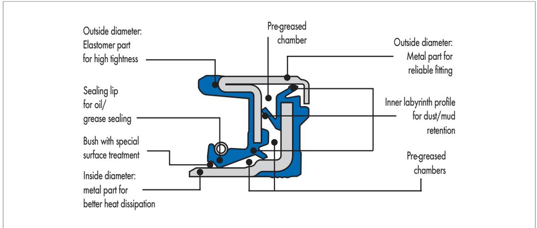
Fig. 41 Simmerring Cassette Seal HS (high speed)
