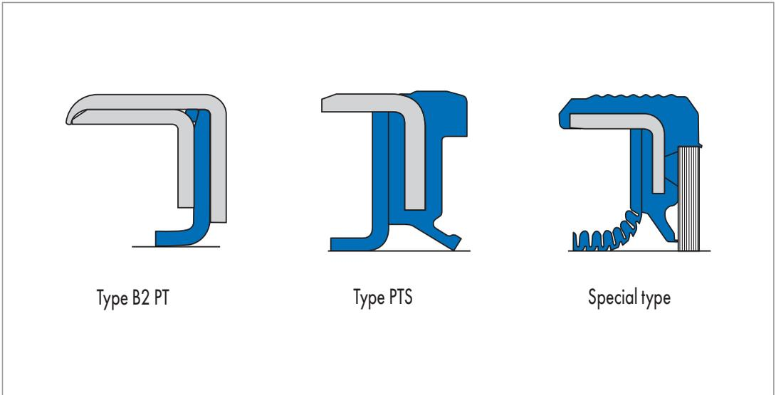
Fig. 36 Simmerrings with PTFE sealing lip
