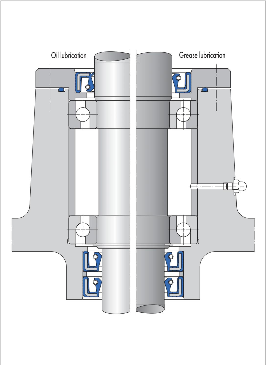
Fig. 6 Sealing of a vertical shaft
