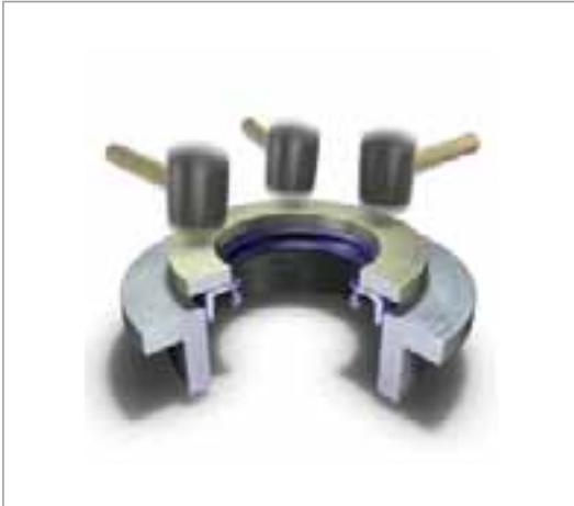
Fig. 49 Permissible hammer assembly
