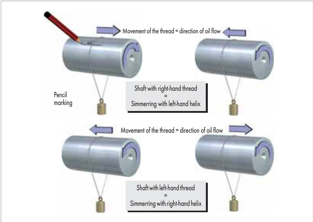
Fig. 30 Determining lead on the shaft
