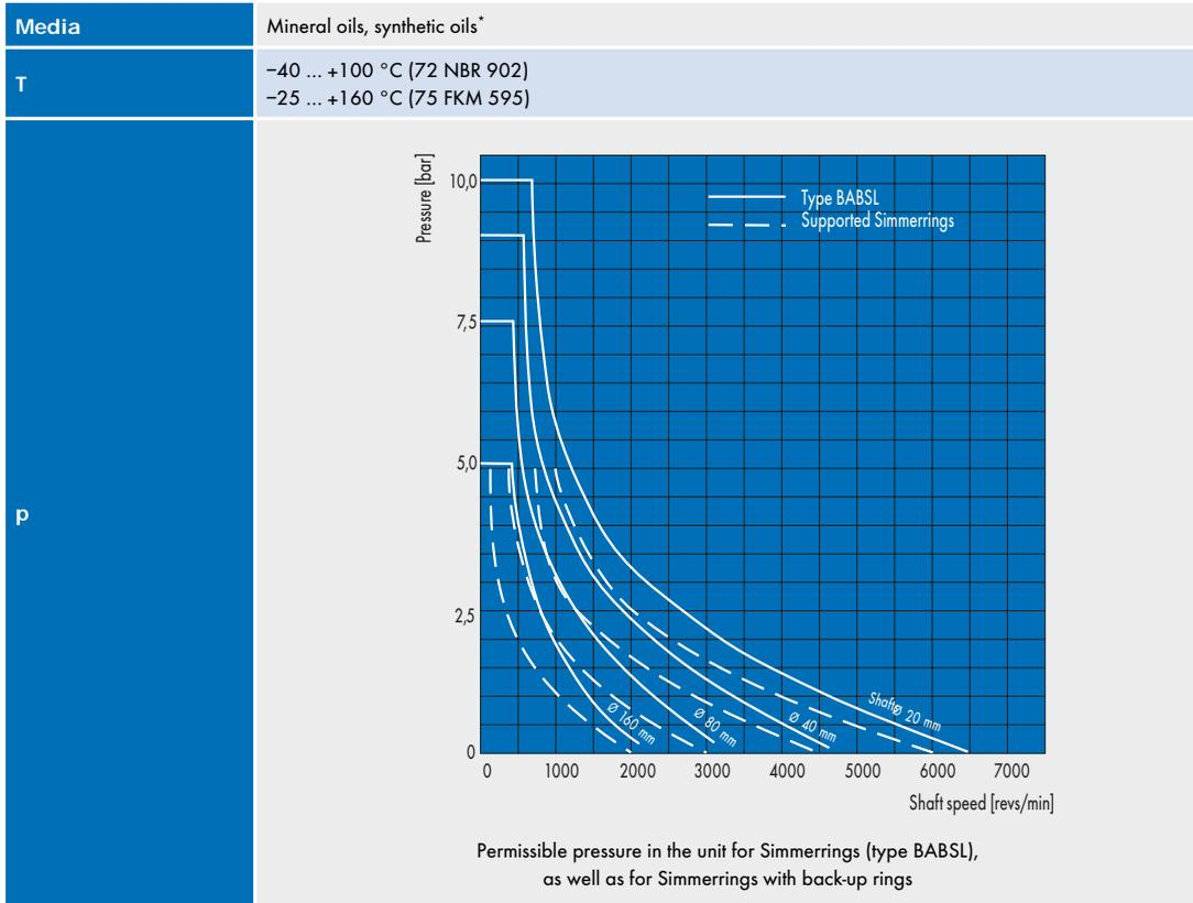
\* With synthetic oils (polyalkylene glycols/polyalphaolefins) it is to be noted that the maximum operating temperature of 80 °C must not be exceeded (only for use of NBR).
