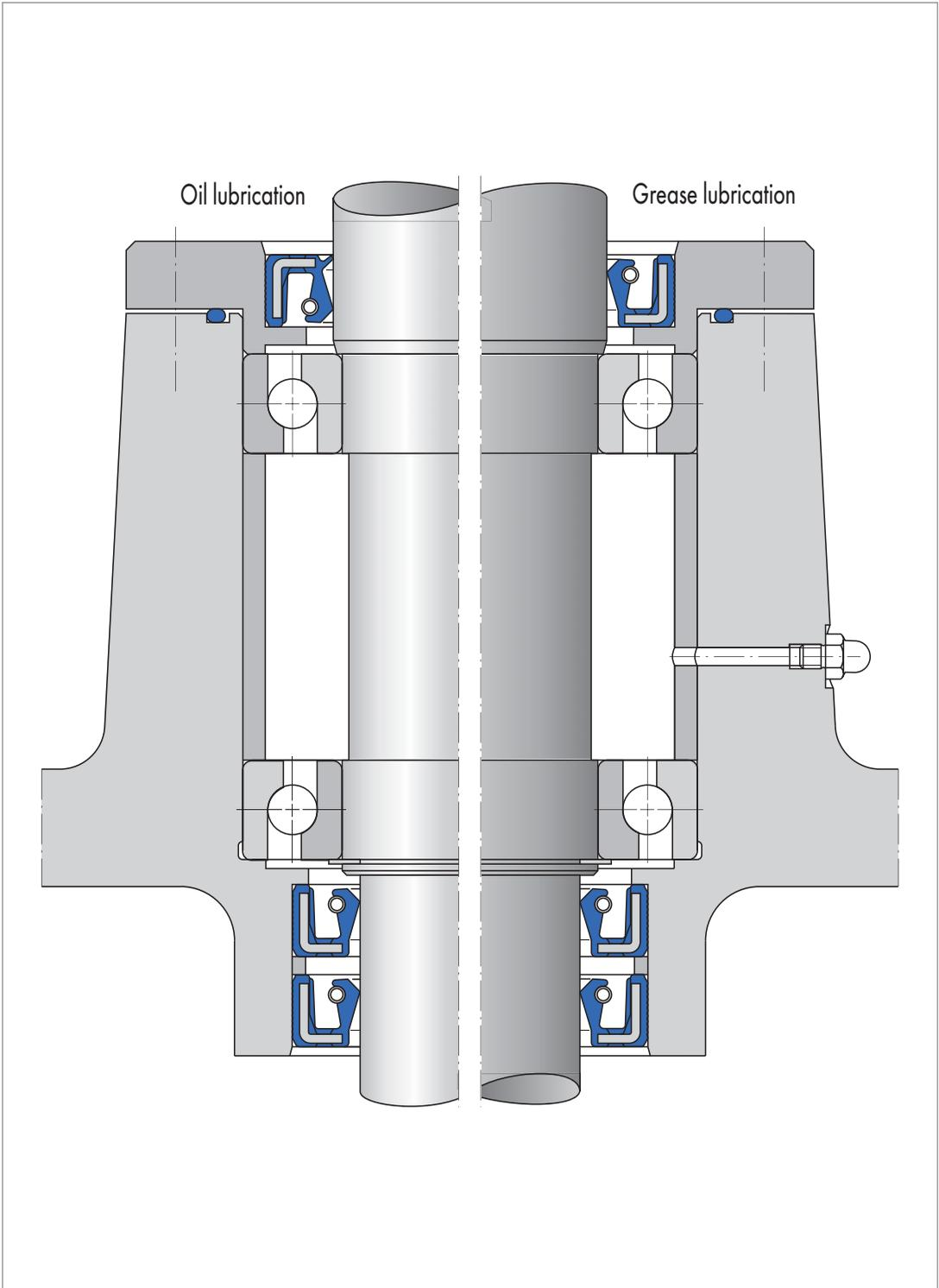
Fig. 6 Sealing of a vertical shaft
