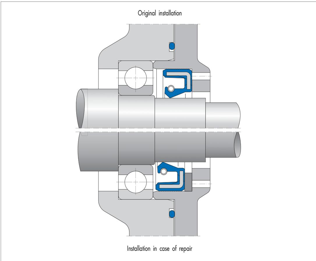
Fig. 52 Fitting on the repair and unit assembly
