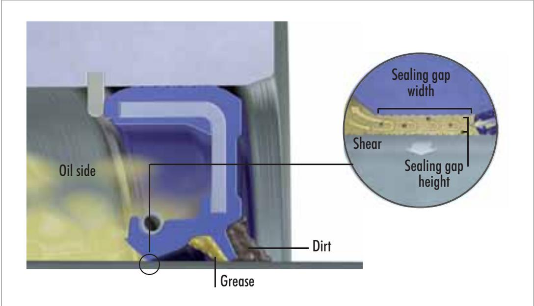
Fig. 10 Simmerring® seal-shaft contact area
