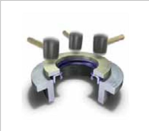
Fig. 49 Permissible hammer assembly
