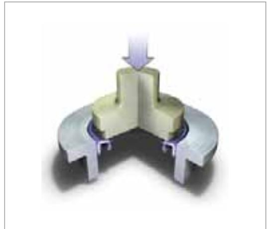
Fig. 48 Diameter of assembly press too small
