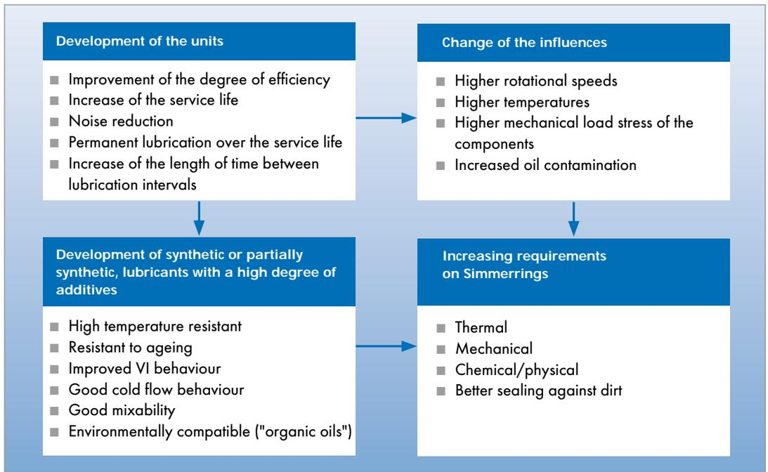
Fig. 18 Increasing requirements on Simmerrings
