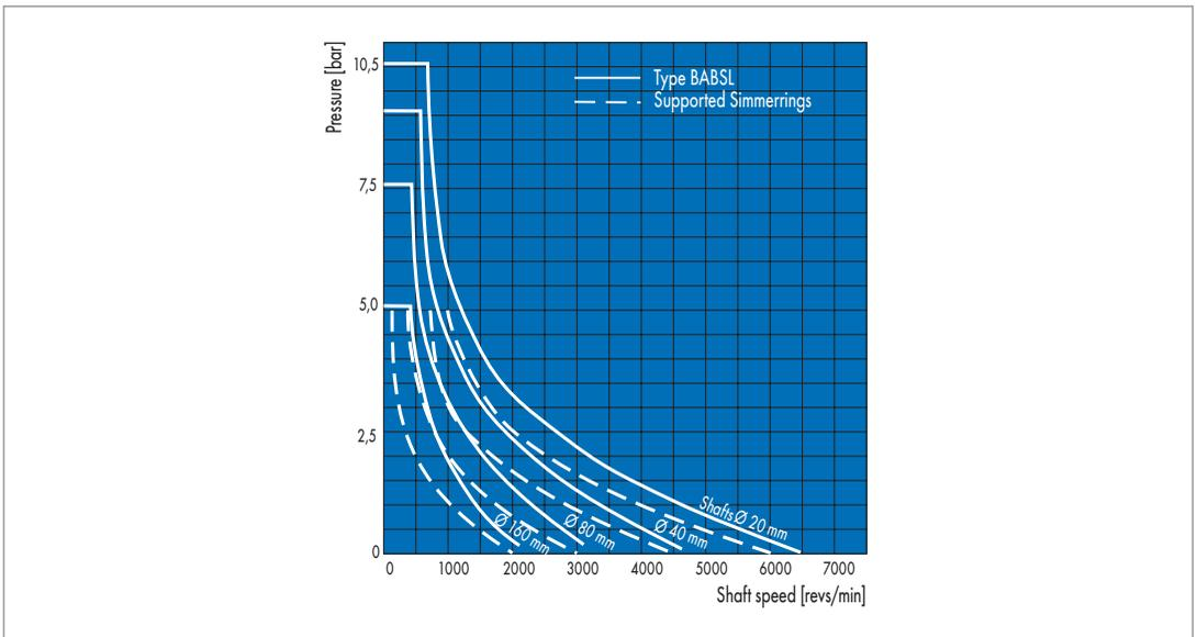
Permissible pressure in the unit for Simmerrings (type BABSL), as well as for Simmerrings with back-up rings.
