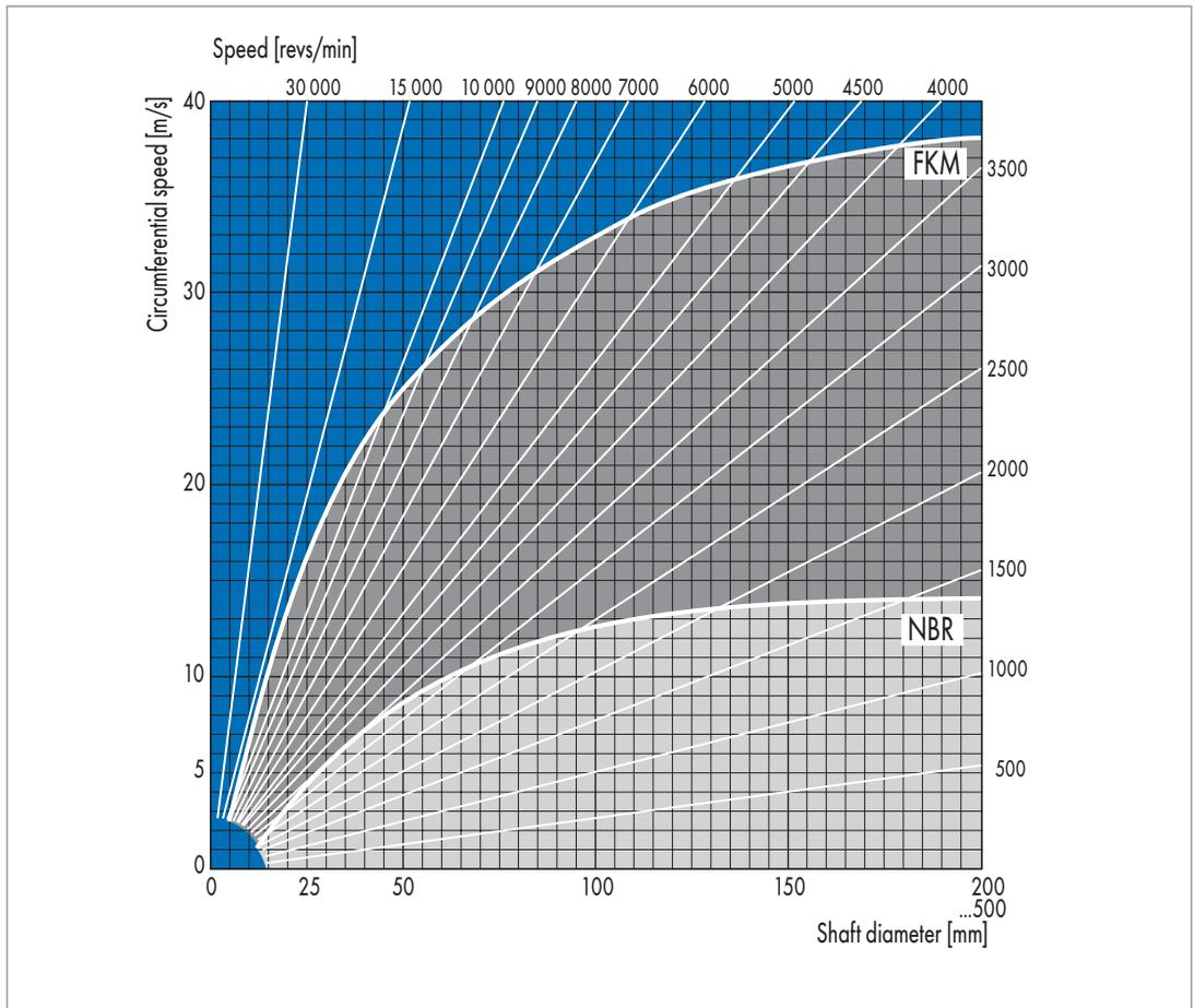
Fig. 20 Permissible circumferential speed for Simmerrings (recommended values) made of the materials NBR (72 NBR 902) and FKM (75 FKM 585) when sealing engine oil SAE 20
