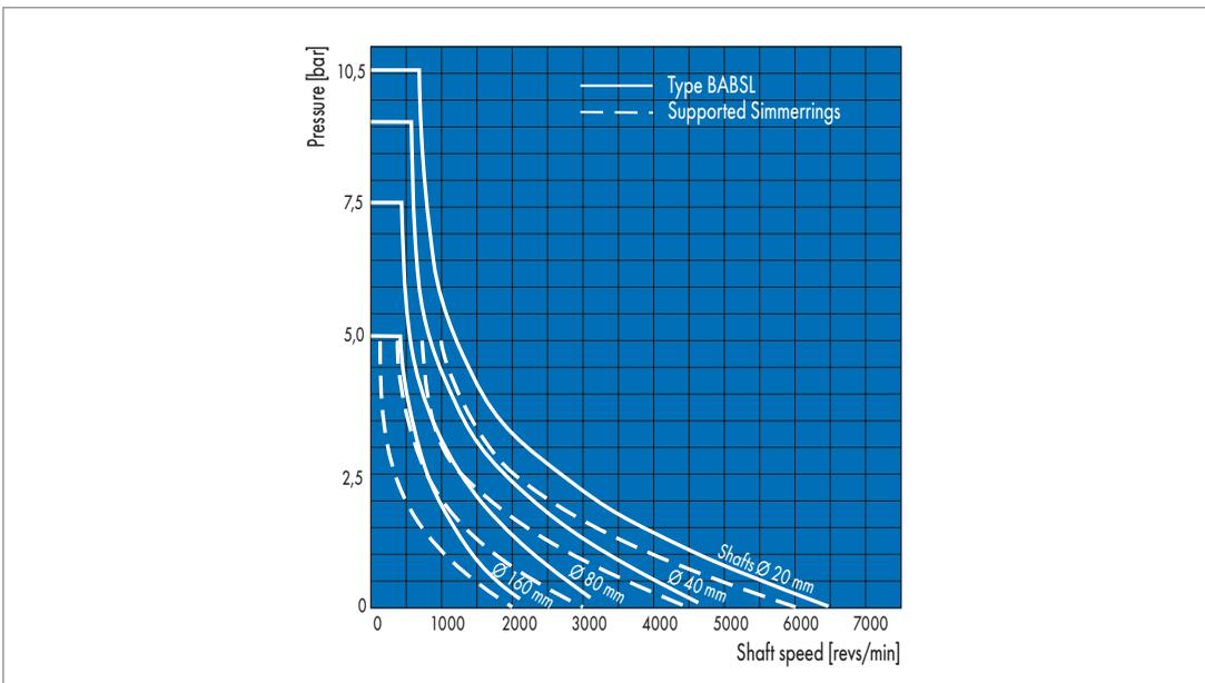
Fig. 25 Permissible pressure in the unit for Simmerrings (Type BABSL), as well as for Simmerrings with back-up rings
