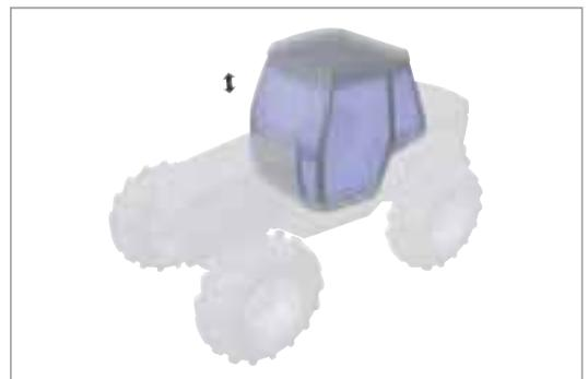
Fig. 6 Vertical vibrations of the cabin after optimisation
